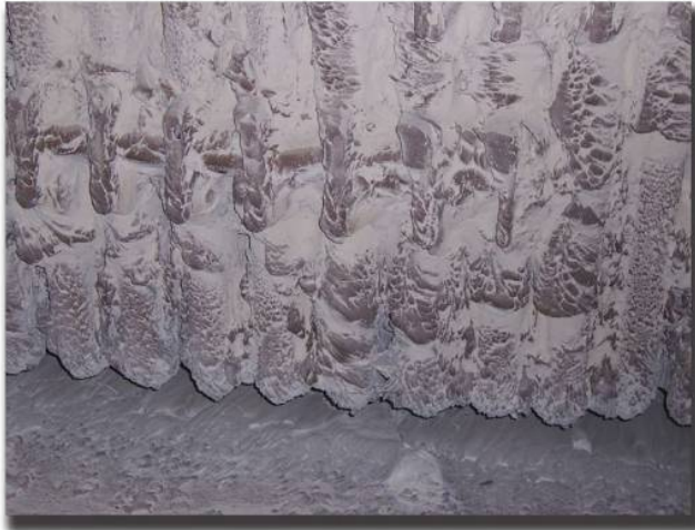
Before being coated, superheater boiler tubes in the Rosebud Operating Services' power plant in Billings experienced severe slag build-up (left) that was removed by sandblasting. After coating the superheater boiler tubes, slag buckles and breaks off (right). Photos courtesy of Dan Gray, Rosebud Operating Services.
